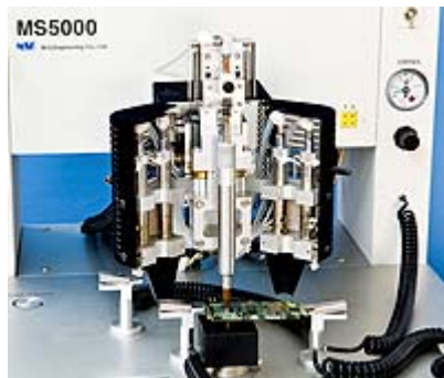
Top heater unit
